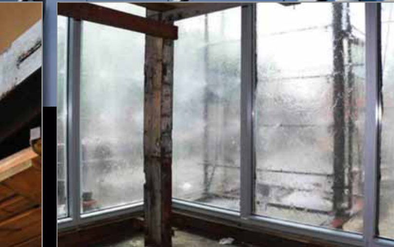
As viewed from the inside of test specimen, a modified static water test is used for field testing the glazing system.
